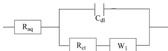
Scheme 2. Equivalent circuit mold for complex impedance plots.  $R_{aq}$ , the solution resistance;  $C_{dl}$ , the modified layer/solution interface capacitance;  $R_{ct}$ , the electron transfer resistance due to the electron transfer at the modified layer/solution interface;  $W_1$ , Warburg diffusion impedance due to the diffusion of the redox couple ( $[Fe(CN)_6]^{4-}/[Fe(CN)_6]^{3-}$ ) in the solution.
