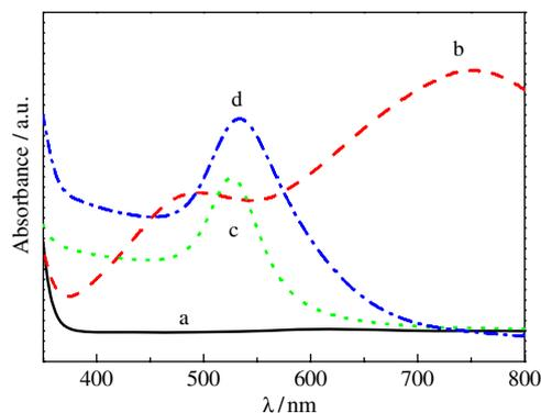
**Figure 1.** UV–vis spectra of (a) 5 mM PTA, (b) a 5 mM mixture of PTA and AA at pH 5.0, (c) 1 mM  $\text{AuCl}_4^-$  at 100 °C and (d) 1 mM  $\text{AuCl}_4^-$  at 20 °C after added such a mixture of PTA and AA.
