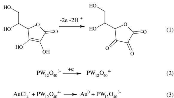
**Scheme 1.** Description of the redox reaction of L-ascorbic acid, PTA and  $\text{AuCl}_4^-$ .
