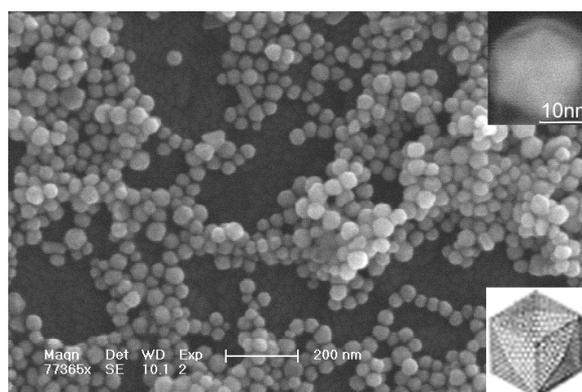
**Figure 3.** Low-magnification SEM image of polyhedral Au nanoparticles prepared at 100 °C (in the upper inset, an enlarged TEM image shows that the polyhedral Au nanoparticles are icosahedral structures, with a typical geometric icosahedron in the lower inset).
