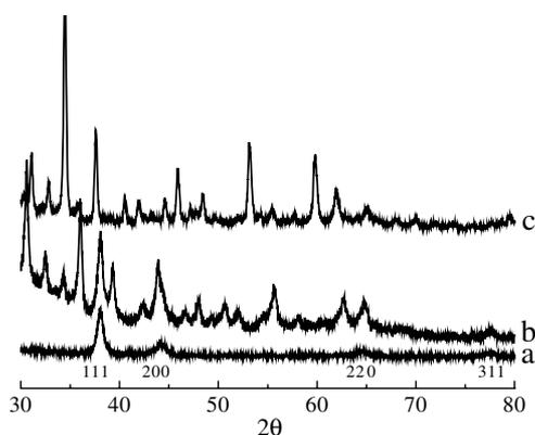
**Figure 5.** XRD patterns recorded from (A) Au, (B) drop-cast film of PTA-gold colloid solution after dialysis and (C) PTA.
