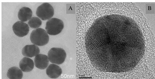
**Figure 4.** (A) TEM image of spherical Au nanoparticles prepared at 20 °C. (B) High-resolution TEM image of a representative spherical Au nanoparticle prepared at 20 °C.
