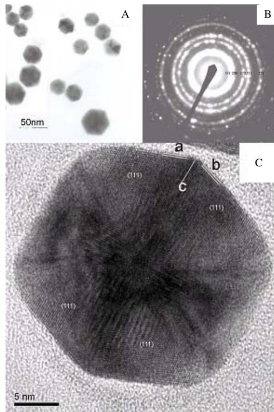
**Figure 2.** (A) TEM image of hexagonal Au nanoparticles prepared at 100 °C. (B) SAED pattern over several hexagonal Au nanoparticles. (C) High-resolution TEM image of a representative hexagonal Au nanoparticle prepared at 100 °C, and the distribution of (111) facets: (a), (b) are labelled as the  $d$ -spacing of a (111) facet, and (c) is labelled as a typical twin boundary between (111) facets.
