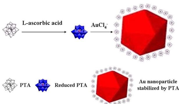
**Scheme 2.** Illustration of the preparation of Au nanoparticles stabilized by PTA.
