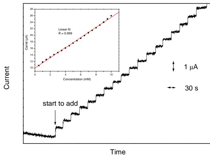
**Figure S3** Amperometric response at the CME-1 to successive addition of  $5.0 \times 10^{-4}$  M  $\text{H}_2\text{O}_2$ . Inserted is the calibration plot. Applied potential: 0.20 V (vs. Ag/AgCl), stirring rate: 300 rpm, supporting electrolyte: phosphate buffer.
