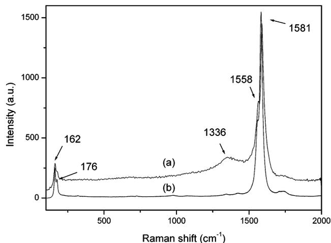
**Figure 1.** Raman spectra of the SWNT-PLL assembly (a) and shortened SWNTs (b).
