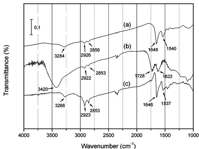
**Figure 2.** FTIR spectra of the SWNT-PLL assembly (a), shortened SWNTs (b), and PLL (c).
