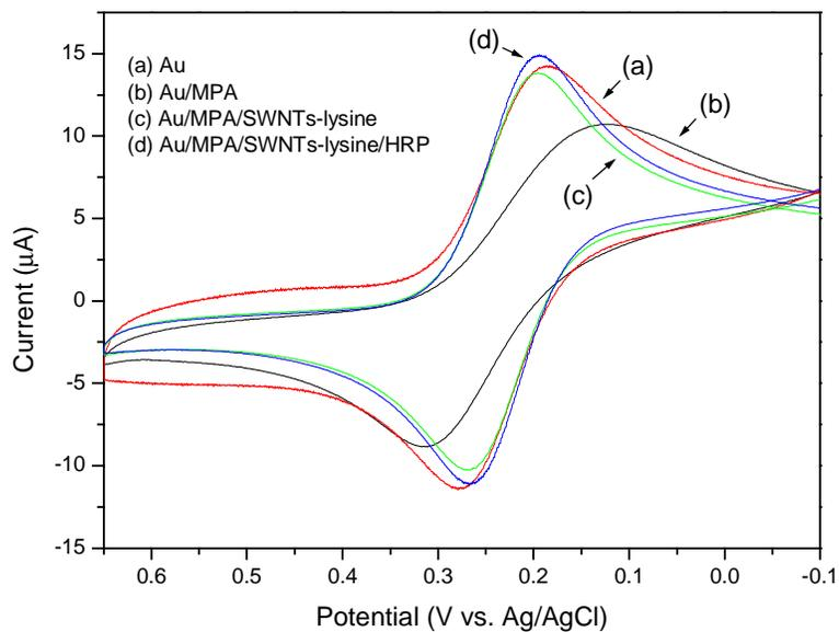
**Figure S2** Cyclic voltammograms of 2 mM  $K_3Fe(CN)_6$  at bare Au (a), Au/MPA (b), Au/MPA/SWNTs-PLL (c) and Au/MPA/SWNTs-PLL/HRP (d) electrode in solution containing 0.1 M KCl as supporting electrolyte. Scan rate: 100 mV/s.
