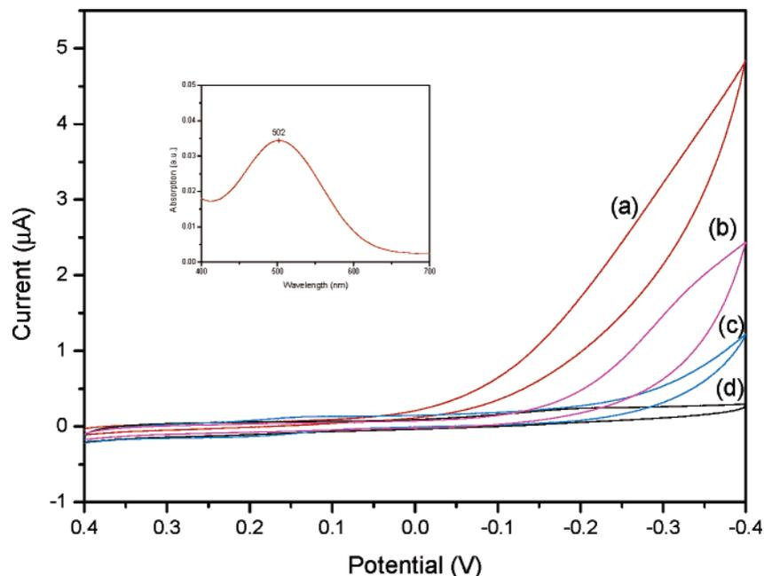
**Figure 3.** Cyclic voltammograms of CME-1 (a), CME-2 (b), the Au/MPA/SWNT-PLL electrode (c) in phosphate buffer (0.05 M, pH 7.4) containing 2.5 mM  $\text{H}_2\text{O}_2$ , and CME-1 (d) in phosphate buffer. Scan rate: 10 mV/s. Inset: UV-vis absorption spectrum of the Trinder reaction by CME-1.
