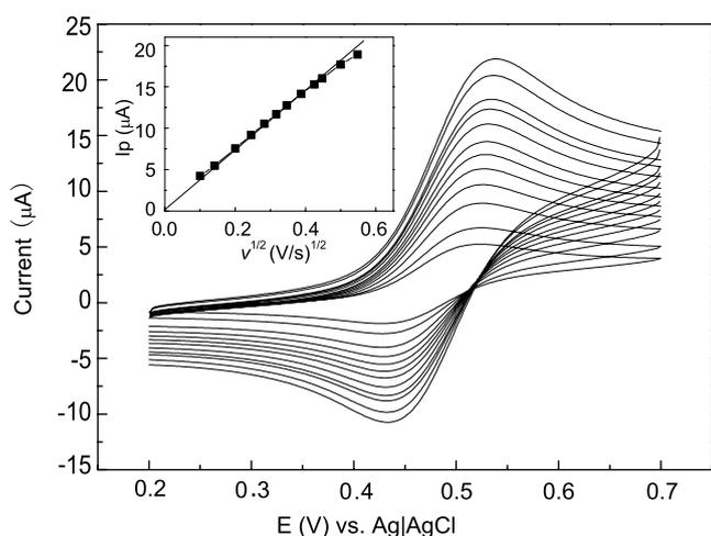
Fig. 4. Cyclic voltammograms of 2 mM FDCA in PBS solution at the GOx/PFIL/sol-gel/GC electrode at scan rates of 0.01, 0.02, 0.04, 0.06, 0.08, 0.1, 0.12, 0.15, 0.18, 0.2, 0.25 and 0.3 V s<sup>-1</sup> (from inner to outer). Inset: the plot of peak current vs. the square root of scan rates.
