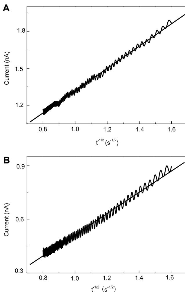
Fig. 5. The plots of current vs.  $t^{-1/2}$  in 2 mM FDCA/PBS solution at the (A) GOx/PFIL/sol-gel/Pt and (B) GOx/sol-gel/Pt microelectrodes, respectively.
