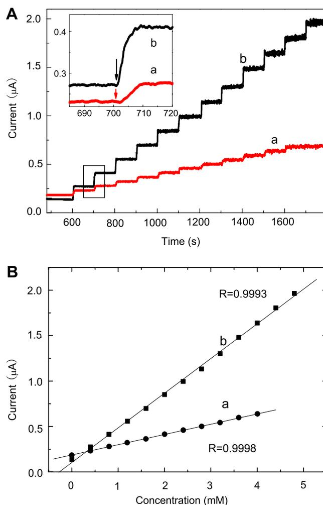
Fig. 1. (A) Steady-state response of (a) GOx/sol-gel/GC and (b) GOx/PFIL/sol-gel/GC electrodes with successive addition of glucose concentration (0.4 mmol/L each step). Applied potential: 1.05 V vs. Ag|AgCl (in saturated KCl). Inset shows a magnification of the second addition of glucose. (B) Calibration curves of the above (a), (b) electrodes.
