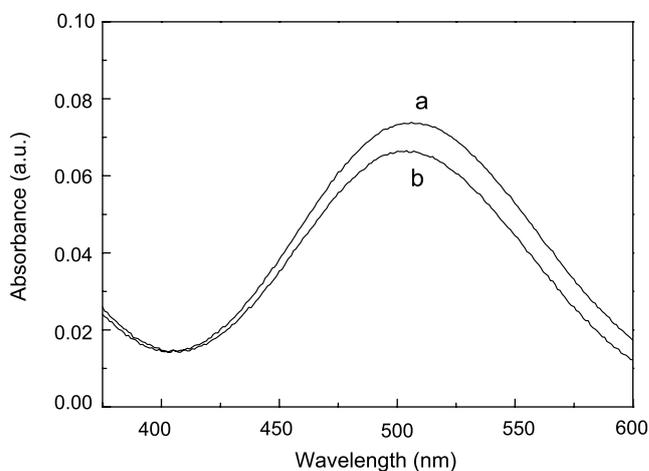
Fig. 6. The enzymatic assay of the immobilized GOx on the PFIL/sol-gel/GC electrode (a) and of the same enzyme electrode after 1 week (b).
