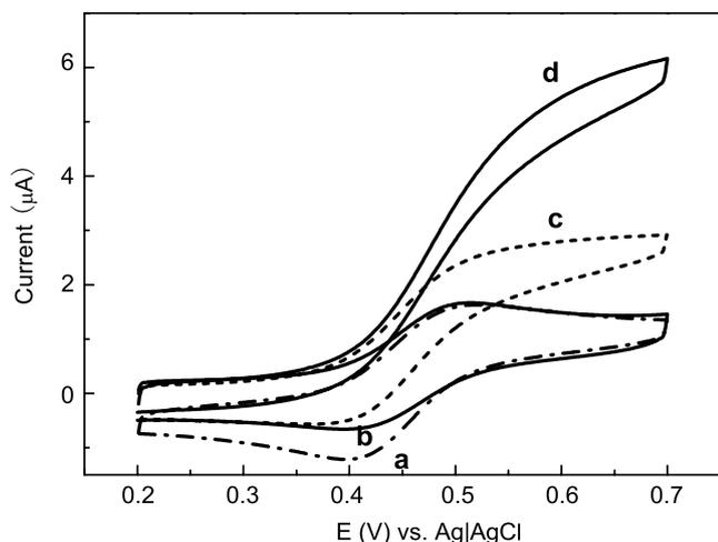
Fig. 2. Cyclic voltammograms of GOx/sol-gel/GC electrode (a and c) and GOx/PFIL/sol-gel/GC electrode (b and d) in 2 mM FDCA/0.1 M PBS solution in the absence (a and b) and presence of 8 mM glucose (c and d), respectively.
