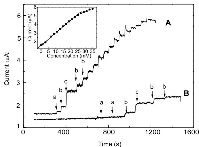
Fig. 3. Current–time response of (A) GOx/PFIL/sol-gel/GC electrode and (B) GOx/sol-gel/GC electrode on injecting (a) 1 mM (b) 2 mM (c) 4 mM of glucose solution under the existence of 2 mM FDCA. Applied potential: 0.55 V. Inset shows a calibration curve at GOx/PFIL/sol-gel/GC electrode.
