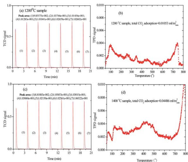
**Fig. 10** Pulsed Adsorption of CO<sub>2</sub> (TCD signal) and Temperature Programmed Desorption (TPD signal) on 1 m<sup>2</sup> (surface area) 1200 °C and 1400 °C SrTiO<sub>3-δ</sub> photocatalyst.
