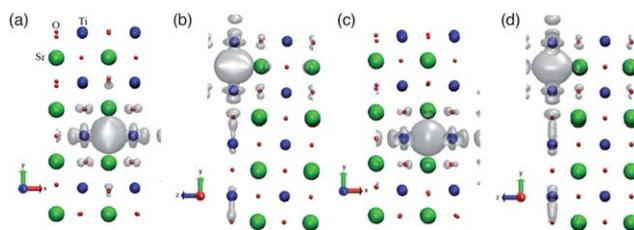
**Fig. 2** Partial charge densities (gray) corresponding to the four occupied states in the band gap at gamma point for model D. Here, green, blue, and red particles denote Sr, Ti, and O atoms, respectively. The isosurface is at 0.01 electrons Å<sup>-3</sup>.
