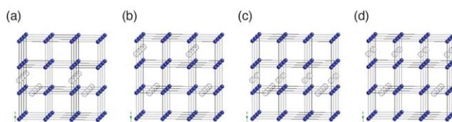
**Fig. 1** Model structures for the reduced SrTiO<sub>3</sub> in which lined oxygen vacancies are placed in different configurations: (a) model A, (b) model B, (c) model C, and (d) model D. These figures are created by extending the 80 atom supercell by 2 × 1 × 2 for the visualization purpose. Blue particles and striped circles represent the positions of Ti atoms and oxygen vacancies, respectively, while Sr and O atoms are not shown in these figures.
