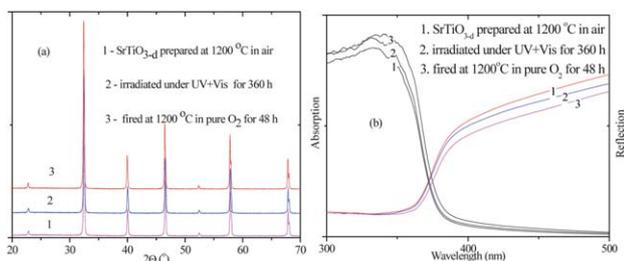
**Fig. 4** XRD and UV-vis spectra of the  $\text{SrTiO}_{3-\delta}$  sample (1) prepared at 1200 °C in air; (2) then illuminated under UV + vis for 360 h in air and (3) fired in pure  $\text{O}_2$  for 48 h.
