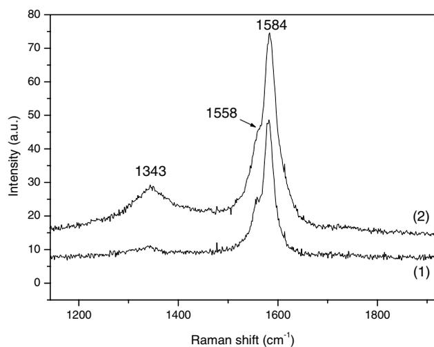
Fig. 4. Raman spectra of SWNTs (curve 1) and SWNTs-PB (curve 2).
