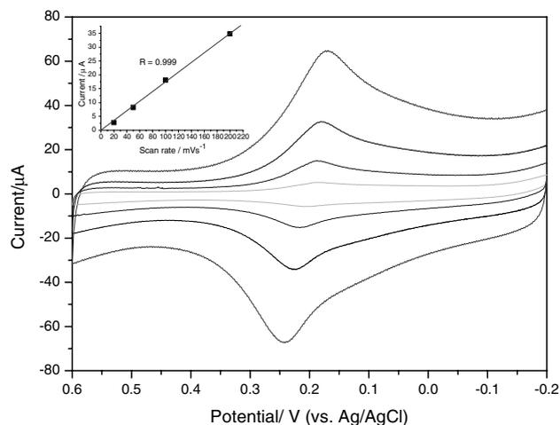
Fig. 5. Cyclic voltammetry of SWNTs–PB modified GC electrode at different scan rates. Inserted is the plot of peak current versus the scan rate. Scan rate: 20, 50, 100, 200 mV/s from inner to outer. Supporting electrolyte: 0.1 M  $K_2SO_4$  solution.
