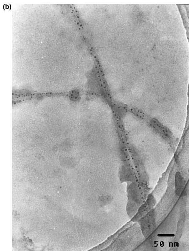
Fig. 1. (a) UV-vis spectra of SWNTs (curve 1), PB (curve 2), and SWNTs-PB (curve 3). (b) TEM image of SWNTs-PB.
