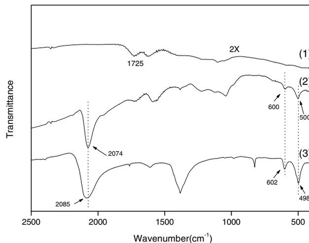
Fig. 2. FTIR of SWNTs (curve 1), SWNTs-PB (curve 2) and PB (curve 3).
