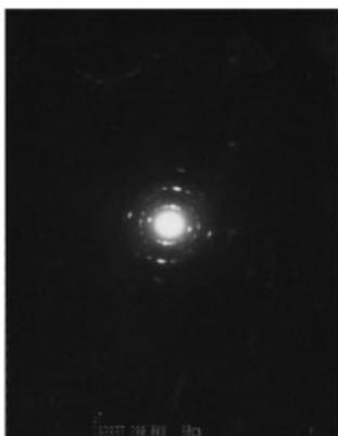
Figure 3 ED pattern of CoHCF nanoparticles.
