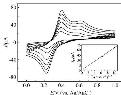
**Figure 10** Cyclic voltammograms of  $2.85 \text{ mmol}\cdot\text{L}^{-1}$  dopamine oxidation on a CoHCF modified electrode at various scan rates. Scan rate ( $\text{mV}\cdot\text{s}^{-1}$ ), 10, 20, 40, 60, 80 and 100. Supporting electrolyte, potassium hydrogen phthalate buffer solution (pH 5.0) containing  $0.1 \text{ mol}\cdot\text{L}^{-1}$  KCl. Inset shows the plot of  $I_{pa}$  vs.  $v^{1/2}$ .
