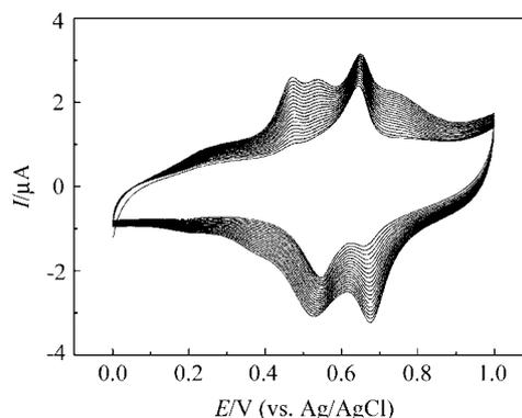
Figure 5 Consecutive cyclic voltammograms of a GC electrode modified with nanosized CoHCF prepared in 0.1  $\text{mol}\cdot\text{L}^{-1}$  KCl solution. Scan rate, 10  $\text{mV}\cdot\text{s}^{-1}$ .
