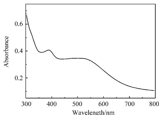
**Figure 1** UV/Vis spectrum of CoHCF in aqueous phase.
