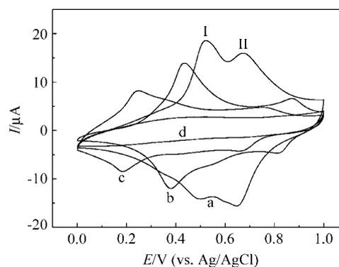
**Figure 7** Cyclic voltammograms of nanosized CoHCF modified electrode in  $0.1 \text{ mol}\cdot\text{L}^{-1}$  KCl (a), NaCl (b), LiCl (c) and  $\text{NH}_4\text{Cl}$  (d) supporting electrolyte solution at a scan rate of  $40 \text{ mV}\cdot\text{s}^{-1}$ .
