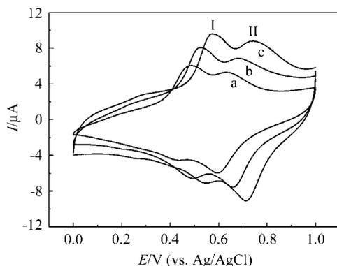
**Figure 8** Cyclic voltammograms of nanosized CoHCF modified electrode in various concentration of KCl solution. (a)  $0.01 \text{ mol}\cdot\text{L}^{-1}$ , (b)  $0.1 \text{ mol}\cdot\text{L}^{-1}$  and (c)  $1.0 \text{ mol}\cdot\text{L}^{-1}$ . Scan rate,  $40 \text{ mV}\cdot\text{s}^{-1}$ .
