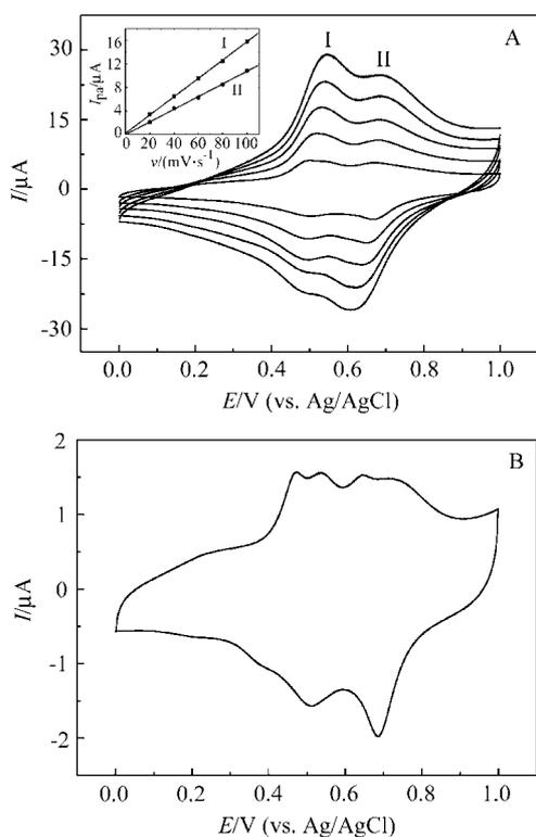
**Figure 6** Cyclic voltammograms of nanosized CoHCF modified electrode in  $0.1 \text{ mol}\cdot\text{L}^{-1}$  KCl solution at various scan rates. Scan rate ( $\text{mV}\cdot\text{s}^{-1}$ ), 20, 40, 60, 80 and 100 in Figure 6A, and 5 in Figure 6B. Inset (A) represents the plots of  $I_{pa}$  vs. scan rates for the redox couples I and II.
