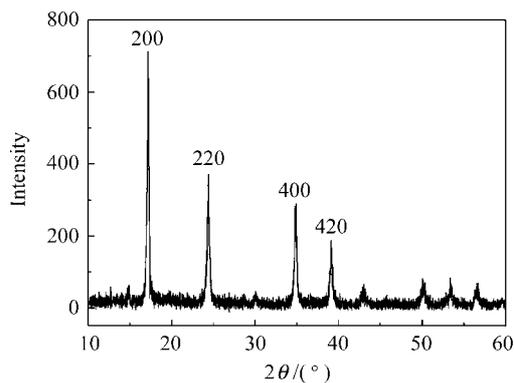
Figure 2 XRD pattern of CoHCF nanoparticles.
