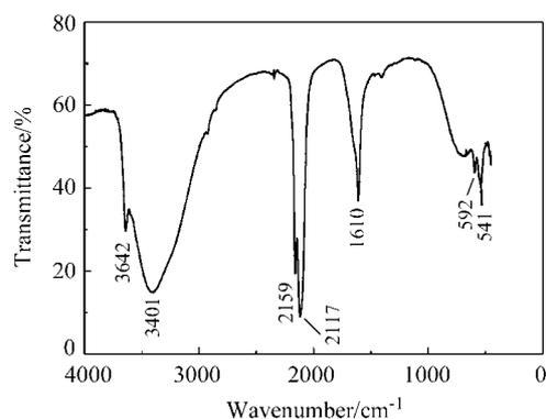
Figure 4 FT-IR spectrum of CoHCF nanoparticles. Several characteristic peaks are labeled.
