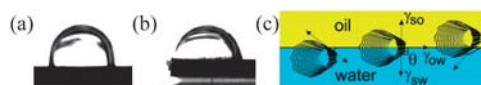
Fig. 3 A water droplet covered with toluene resting on (a) a SWNT-Im film transferred from the W/O interface, and on (b) a SWNT-COOH film by spin-coating on a silicon wafer. (c) Schematic position of a SWNT at the W/O interface for a contact angle less than 90^\circ (left), equal to 90^\circ (middle) and greater than 90^\circ (right).
