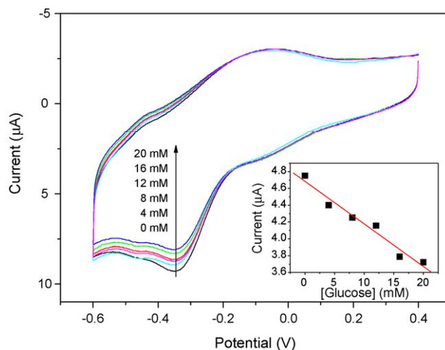
Fig. 5. Cyclic voltammograms at GCE/SWNT-IL-GOD in various concentrations of glucose PBS solution saturated with air: 0, 4, 8, 12, 16, and 20 mM from outer to inner. The inset is the calibration curve corresponding to amperometric responses. Scan rate: 0.05 V s<sup>-1</sup>.
