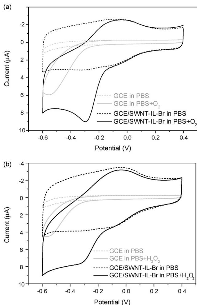
Fig. 4. (a) Cyclic voltammograms at bare GCE (gray) and GCE/SWNT-IL-Br (black) in 0.05 M air saturated (solid) PBS solution and after degassed with pure N<sub>2</sub> (dotted). (b) Cyclic voltammograms at bare GCE (gray) and GCE/SWNT-IL-Br (black) in 0.05 M N<sub>2</sub> saturated PBS solution in the absence (dotted) and in the presence (solid) of 2.5 mM H<sub>2</sub>O<sub>2</sub>. Scan rate: 0.05 V s<sup>-1</sup>.
