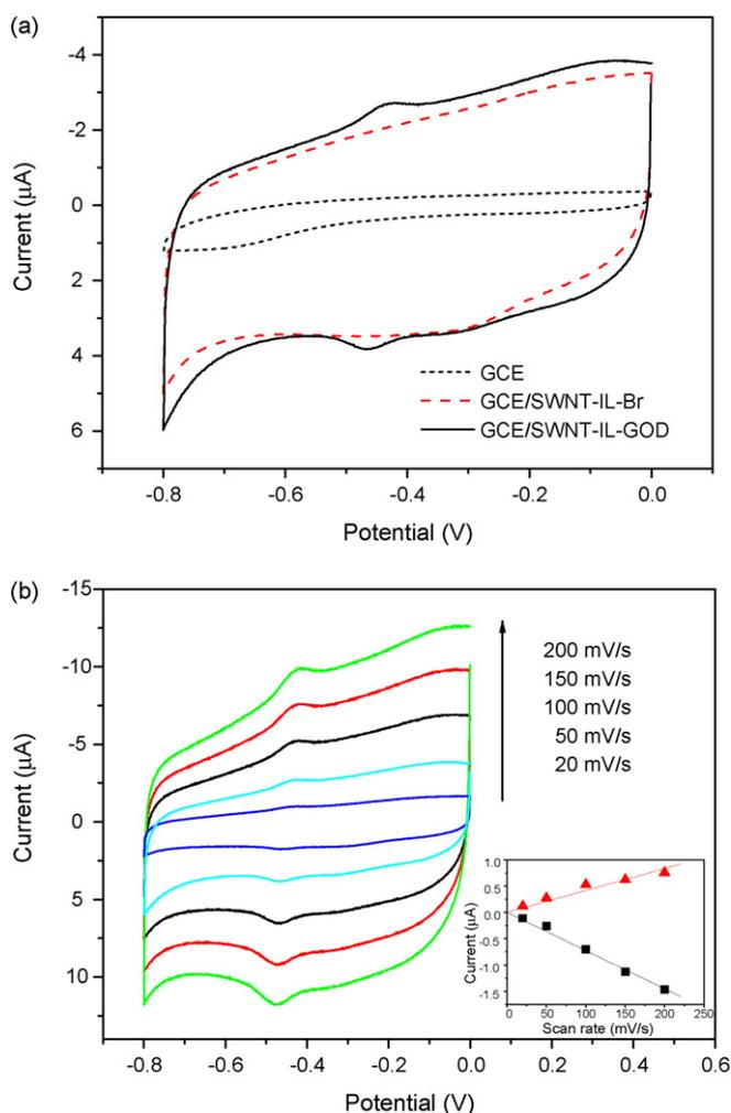
Fig. 2. (a) Cyclic voltammograms at bare GCE (dotted), GCE/SWNT-IL-Br (dashed) and GCE/SWNT-IL-GOD (solid) in 0.05 M  $N_2$  saturated PBS solution (pH 7.4). Scan rate:  $0.05$  V  $s^{-1}$ . (b) Cyclic voltammograms at GCE/SWNT-IL-GOD electrode in 0.05 M  $N_2$  saturated PBS solution at different scan rates. Scan rate: 0.02, 0.05, 0.1, 0.15 and  $0.2$  V  $s^{-1}$  from inner to outer. Inserted is the calibrated plot of peak currents vs. scan rates.
