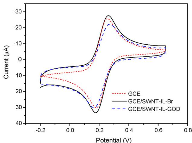
Fig. 1. Cyclic voltammograms of 2 mM  $K_3Fe(CN)_6$  with 0.1 M KCl at bare GCE (dotted), GCE/SWNT-IL-Br (solid) and GCE/SWNT-IL-GOD (dashed).
