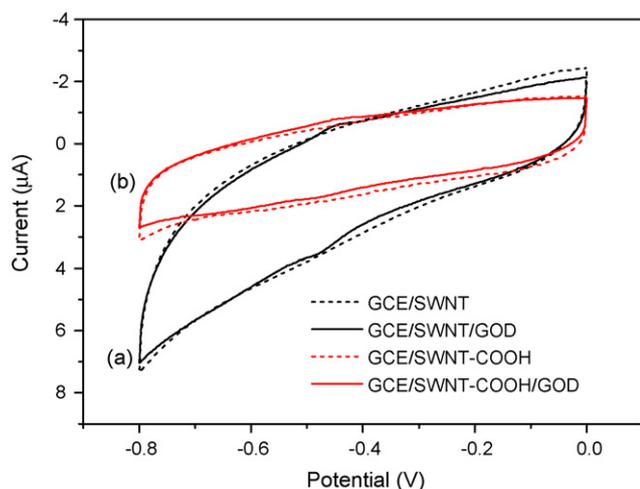
Fig. 3. Cyclic voltammetric measurements at (a) GCE/SWNT (dotted), GCE/SWNT/GOD (solid), (b) GCE/SWNT-COOH (dotted) and GCE/SWNT-COOH/GOD (solid) in 0.05 M  $N_2$  saturated PBS solution (pH 7.4). Scan rate:  $0.05 \text{ V s}^{-1}$ .
