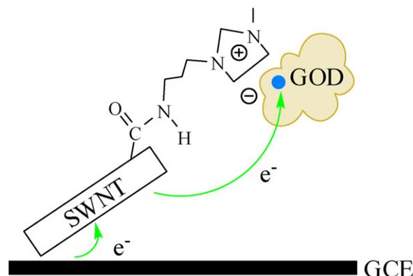
Scheme 1. SWNT-IL-GOD bionanocomposite-modified glassy carbon electrode.
