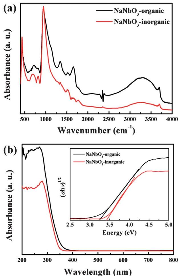
**Fig. 3** (a) FT-IR spectra and (b) UV-vis absorption spectra of  $\text{NaNbO}_3$ -inorganic and  $\text{NaNbO}_3$ -organic. The inset in figure (b) shows the corresponding  $(\alpha h\nu)^{1/2} \sim h\nu$  curves.
